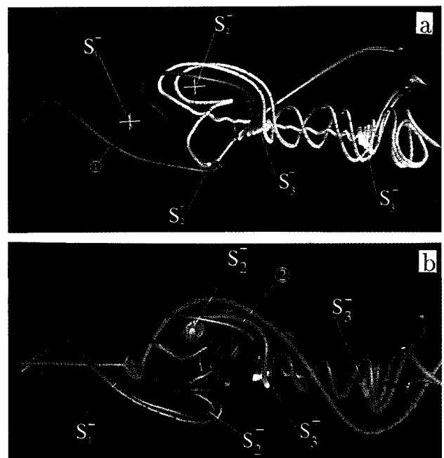
Fig. 13 Three-dimensional critical points and trajectories in vortex breakdown region at t^+ = 2.4 .
